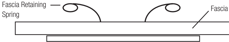
Fig. 3: Fascia retaining springs side view
