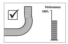
Fig. 10: Gradual bends, ducting stretched straight
