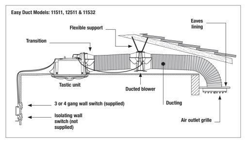
Fig. 4: Layout of Tastic Easy Duct
