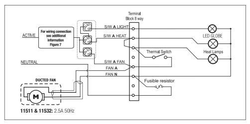
Fig. 5: Wiring diagram for model 11511 & 11532
