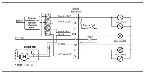
Fig. 6: Wiring diagram for model 12511
