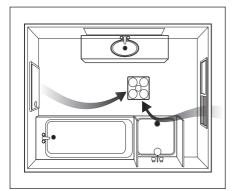
Fig. 1: Ideal placement of Tastic. Sufficient air inlets into room are required
