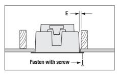
Fig. 3: Joist clearances
