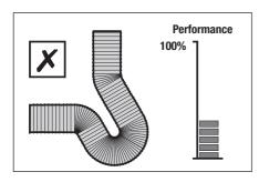
Fig. 11: Tightly compressed bends
