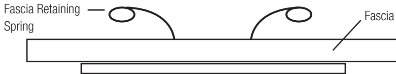
Fig. 3: Fascia retaining springs side view
